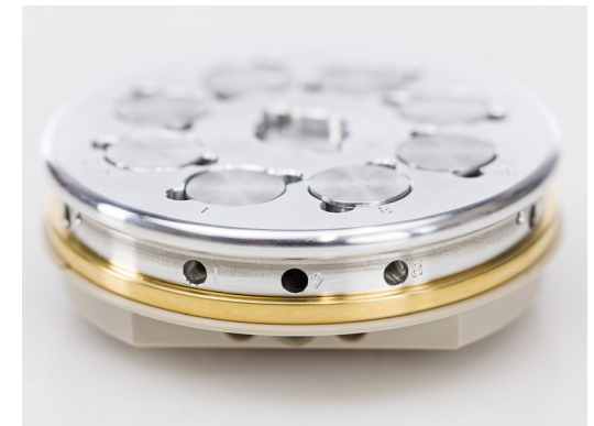
Tandem decel sample holder for 9 single specimens.
