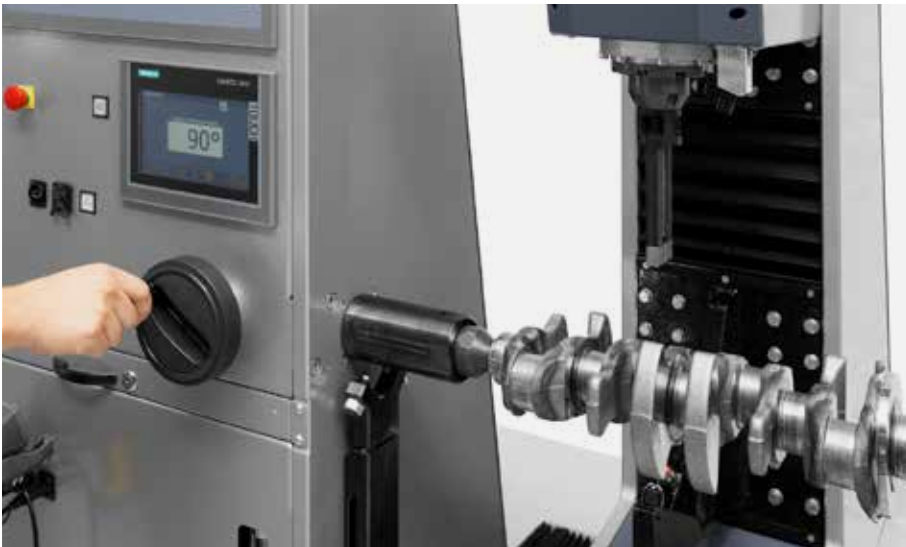
HARDNESS TESTING OF CRANKSHAFTS
