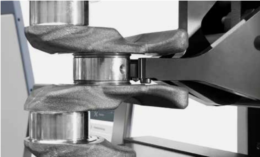
INDENTOR EXTENSION FOR HARD-TO-REACH TEST LOCATIONS
