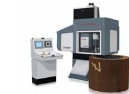
MILLING AND HARDNESS TESTING POSITION
